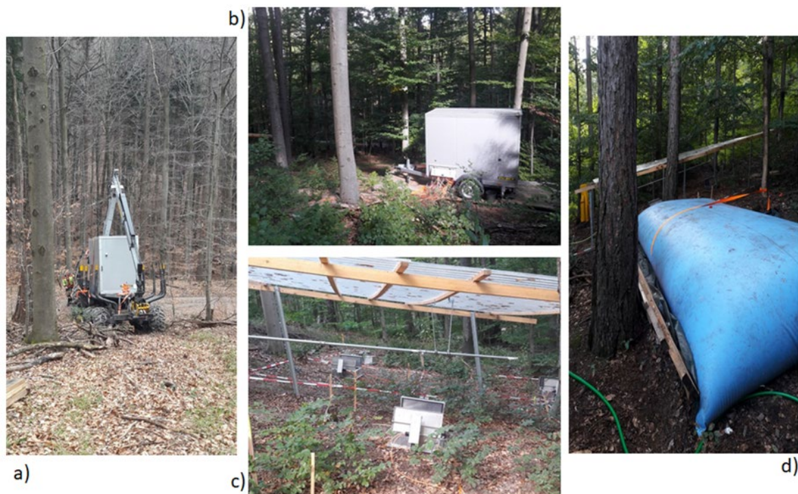
Figure 18. Transport of the GasFluxTrailer to the plots (a) GasFluxTrailer on site (b) automated gas chambers and rain-out shelter (c), and water reservoir for the rewetting experiment (d) at Klausenleopoldsdorf. Source: B. Kitzler, 2021
